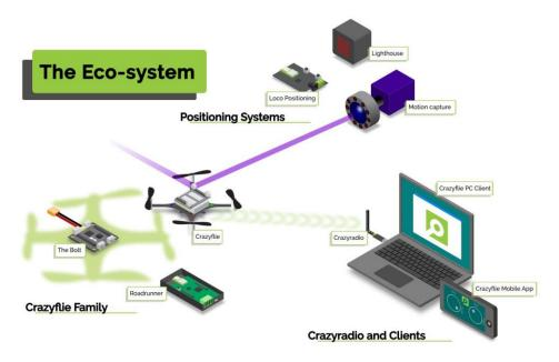
The compilation requires a wired connected with a computer, with the quadrotor in the bootloader mode. A Crazyflie can communicate with a phone or PC using BLE, when **flying manually with the Crazyflie companion app** or **custom designs**. Additionally, a custom USB dongle called Crazyradio PA, or Crazyradio for short, allows **lower latency communication**. The radio communication use a proprietary protocol, the **Crazy RealTime Protocol** (CRTP).
